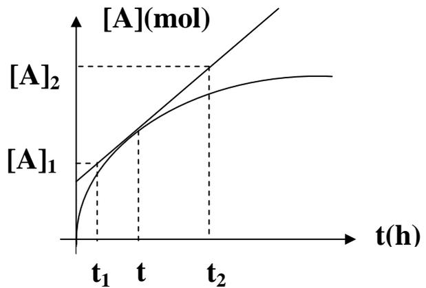
$$v_A = \frac{[A]_2 - [A]_1}{t_2 - t_1}$$
