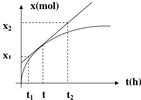
$$v = \frac{1}{V} \frac{x_2 - x_1}{t_2 - t_1}$$
