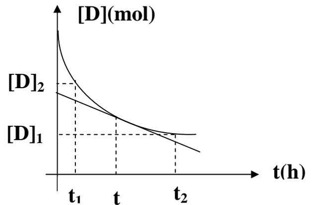
$$v_D = -\frac{[D]_2 - [D]_1}{t_2 - t_1}$$
